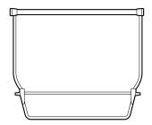
The cargo cover is a retractable cover that is available as an option for all R1S trim levels. You can use it to shade your cargo from damaging ultraviolet rays or to obscure your cargo.
