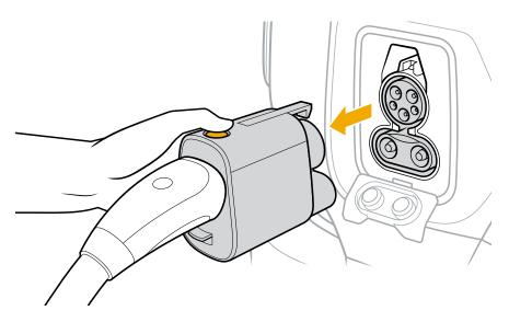
4. Press down on the tab below the NACS adapter port and pull the charge plug out of the adapter.
