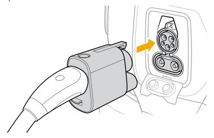
3. When charging is complete, press the button on the top of the adapter to release the latch, and remove the plug with adapter from the vehicle.
